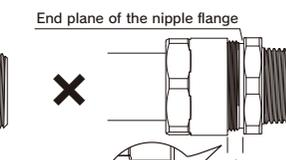
**Warning** Tighten the hexagonal cap nut completely until it touches the flange of the nipple to prevent the hose from becoming detached and the fluid from leaking.
